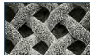
After sandblasting, bracket base is more porous, increasing bond strength
